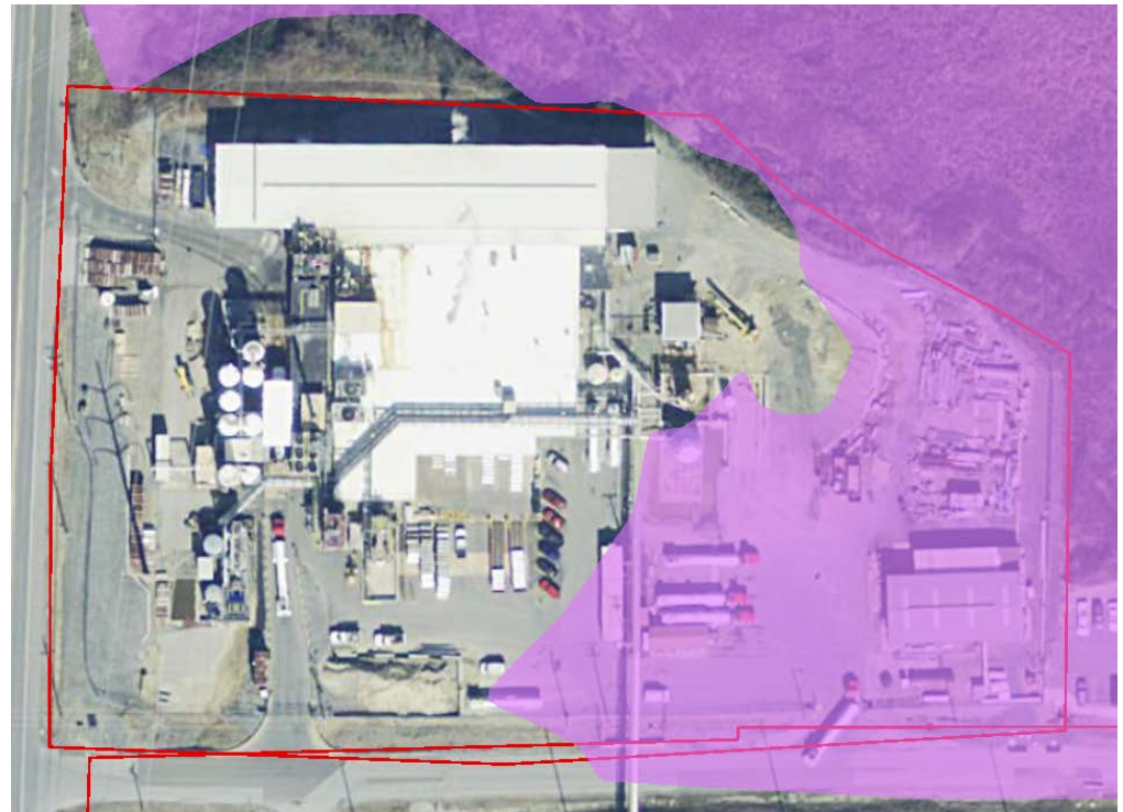
Chloramone site. Purple indicates inundation area of 1% storm and sea level rise combined from FRAM.
