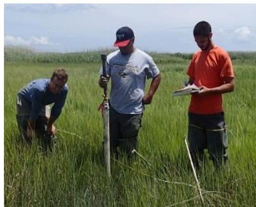
Figure 9. DNREC scientists measure bearing capacity, an indicator of marsh stability, in a tidal marsh using a slide hammer during a site assessment.
