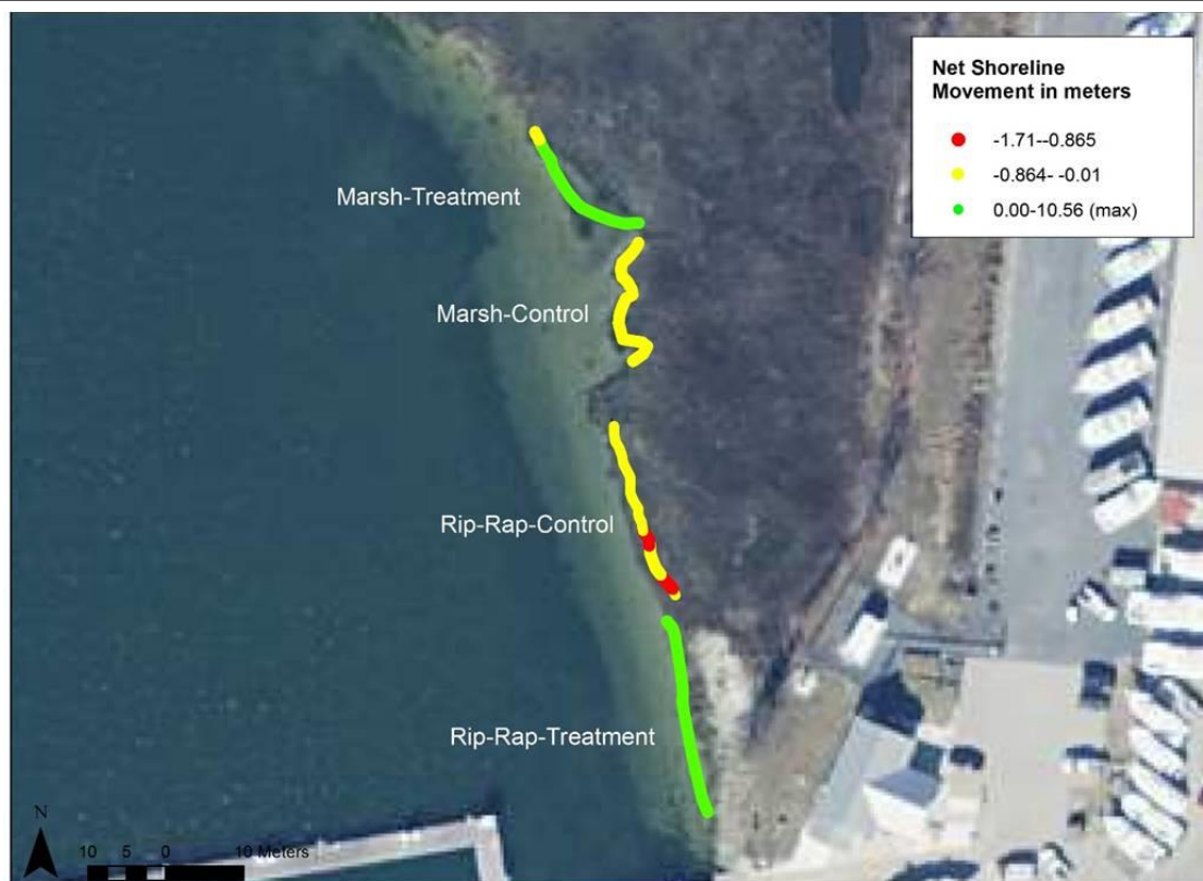
Figure 15 Net Shoreline Movement is overall movement of the shoreline between the oldest shoreline measurement and the most recent shoreline measurement. Areas in green reflect a net waterward shoreline movement (i.e. gain of marsh area). Red and yellow represent areas where there was net landward shoreline movement (i.e. loss of marsh area). The difference in red and yellow was based on the mean of the overall net shoreline movements across all sites.
