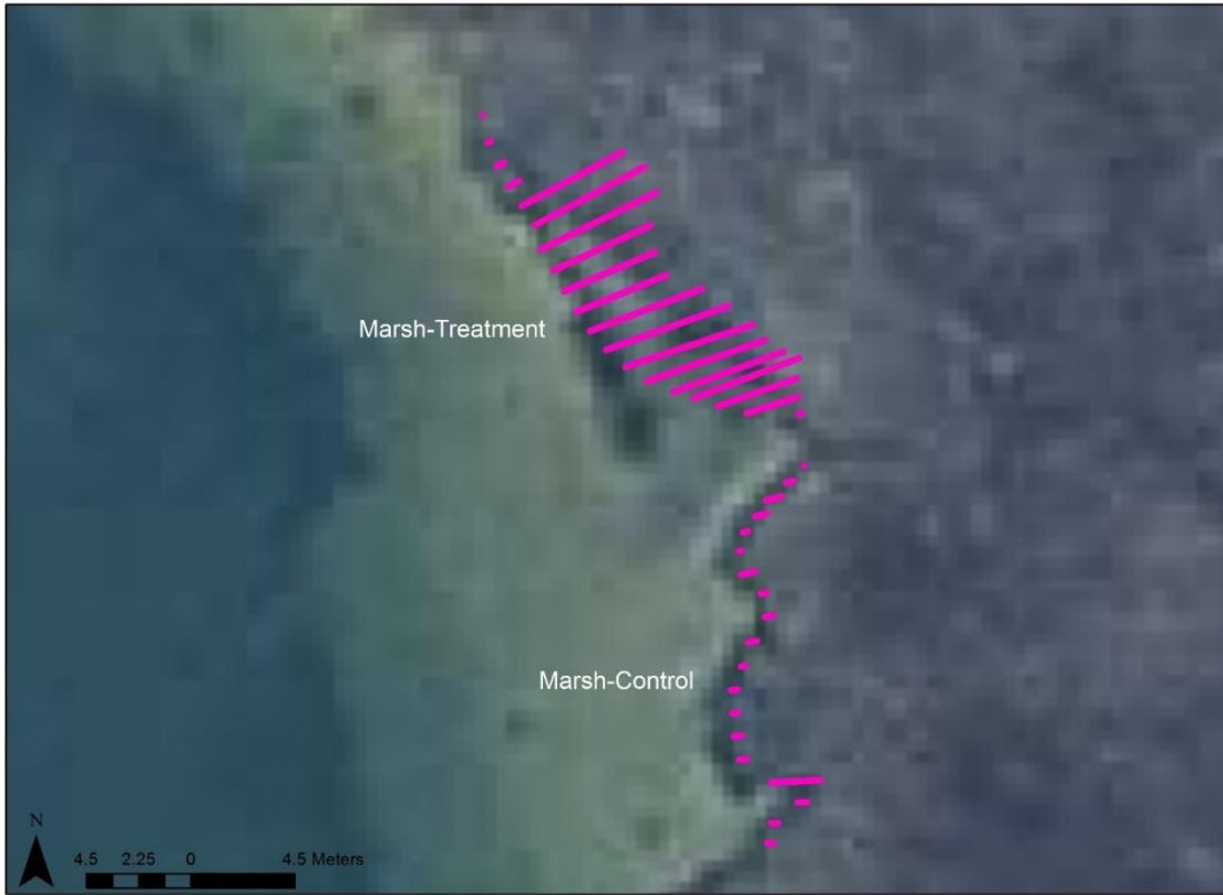
Figure C3. Transect locations and lengths (between most waterward and landward vegetation lines) generated from DSAS for the Inland Bays Marsh study location.
