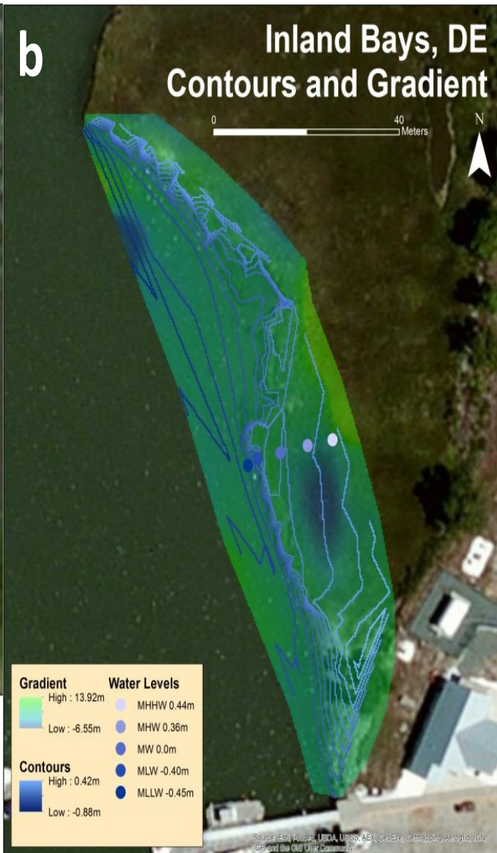
Figure 6 Contour and gradient profiles along the Lewes (a) and Inland Bays (b) locations. Contour lines and gradient polygon spanned the area between mean lower low water and mean higher high water. Local tidal datum elevation represented as points.
