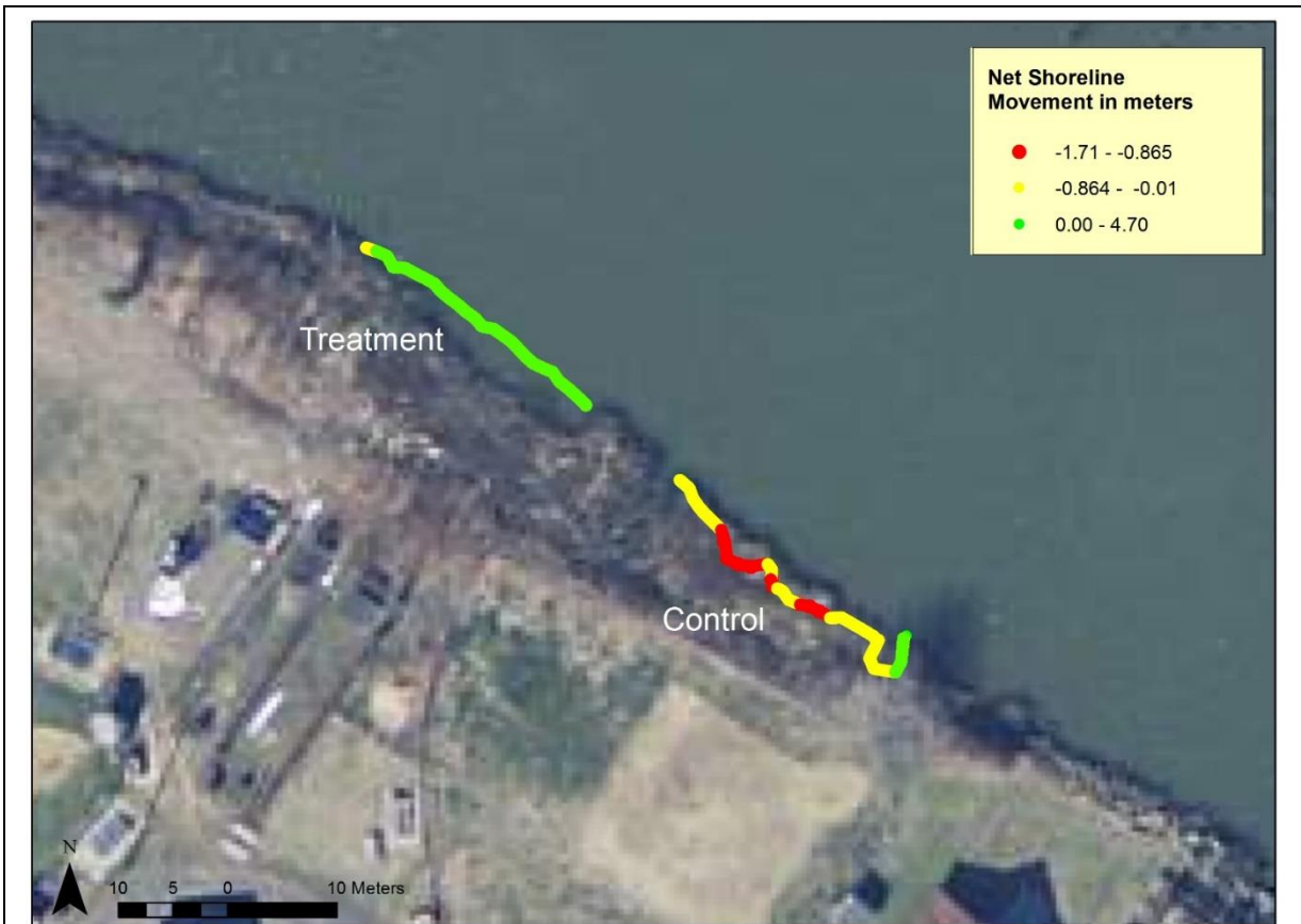
Figure 11 Net Shoreline Movement is overall movement of the shoreline between the oldest shoreline measurement and the most recent shoreline measurement. Areas in green reflect a net waterward shoreline movement (i.e. gain of marsh area). Red and yellow represent areas where there was net landward shoreline movement (i.e. loss of marsh area). The difference in red and yellow was based on the mean of the overall net shoreline movements across all sites. The area at the end of the control shoreline, although showing positive movement, upon closer inspection, was most likely caused by a mis-measurement by DSAS transects around a curve.
