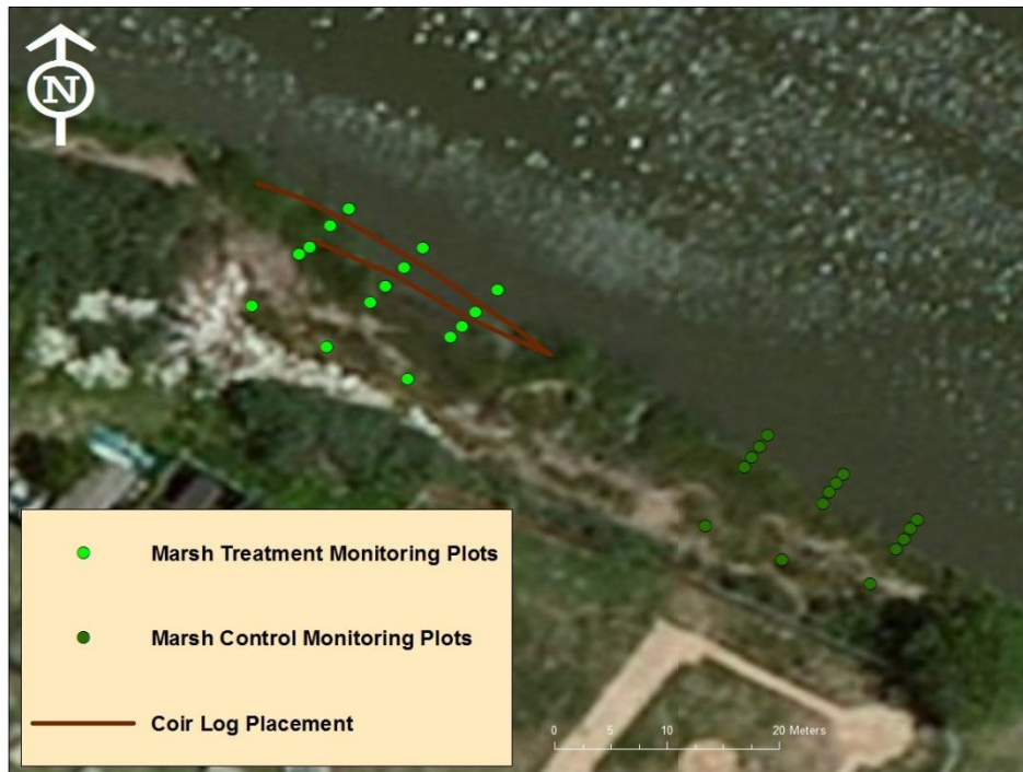
Figure 9 Position of monitoring plots and coir log treatments within the paired treatment and control areas at the Lewes living shoreline location. Monitoring plot locations and log positions collected using RTK-GPS.
