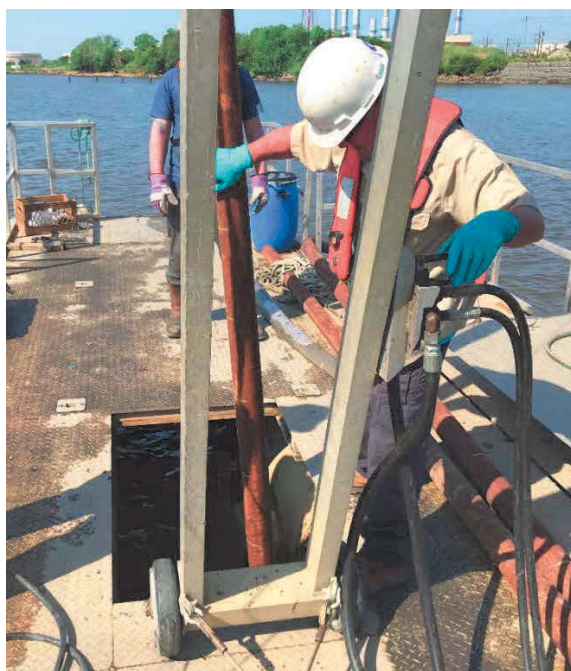
Photo 3. Collection of Vibracore in Delaware River through Hatch
