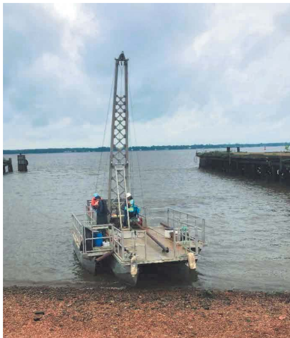
Photo 2. Pontoon Mounted Vibracore Rig
