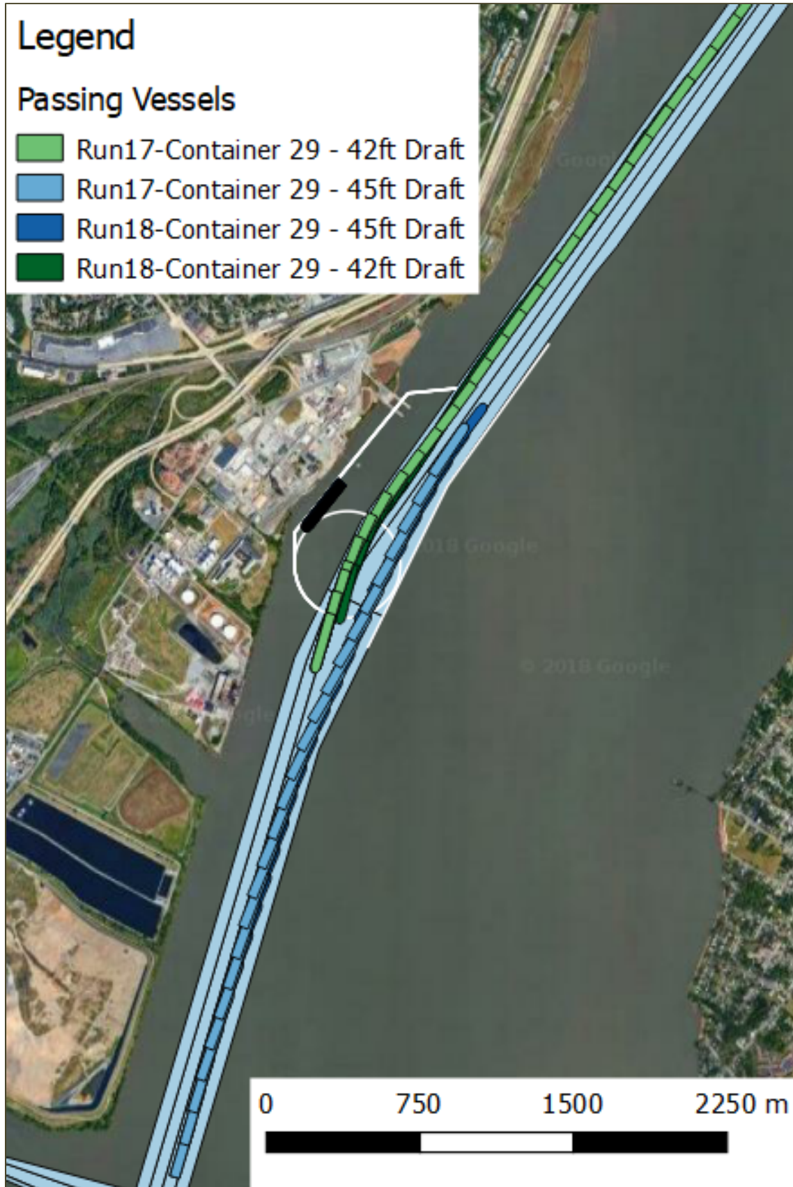
Figure 4-9: Passing vessels – maximum flood current, 25 kts wind from 90°
