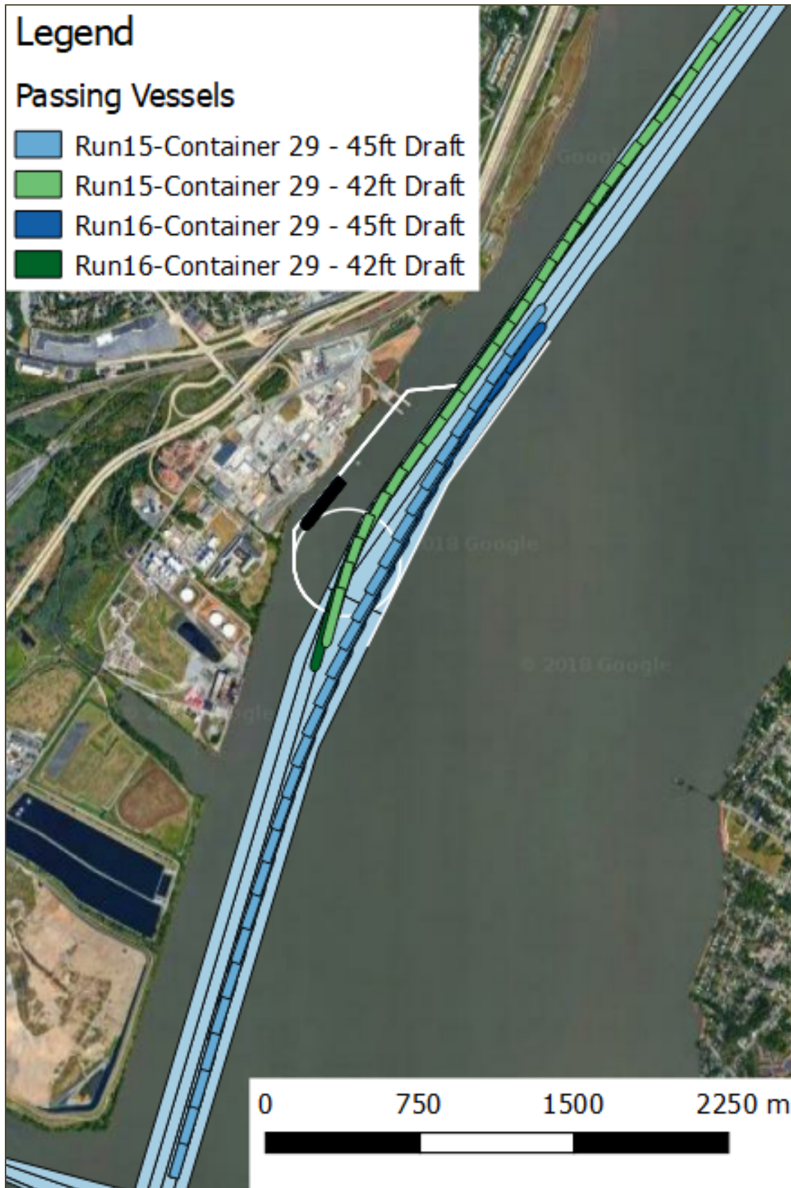
Figure 4-8: Passing vessels – maximum flood current, 25 kts wind from 135°
