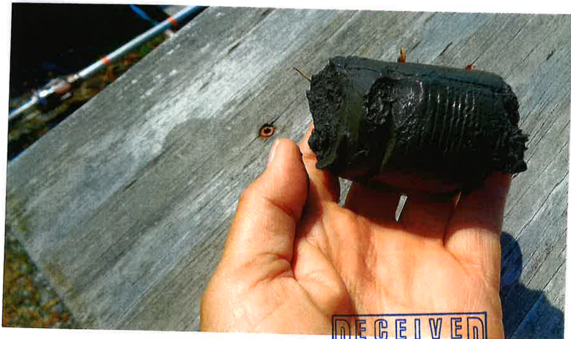
Figure 11. Photographs of sediment core from Bay Vista Marina basin. Material consists predominantly of mud (silt + clay).
