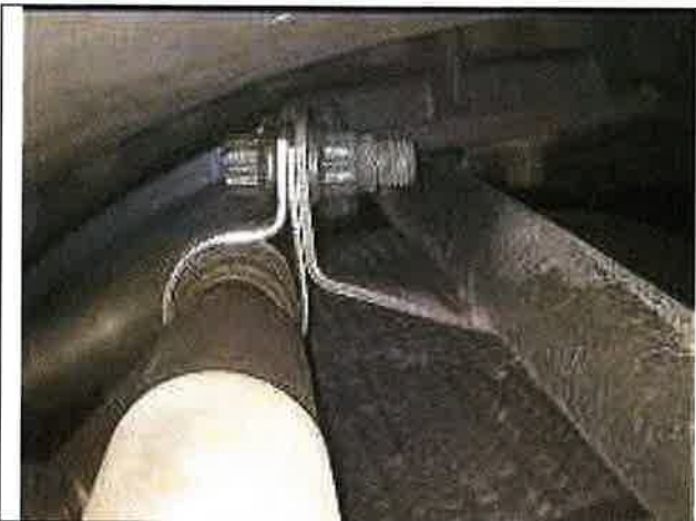
CRF Manifold Clamping
