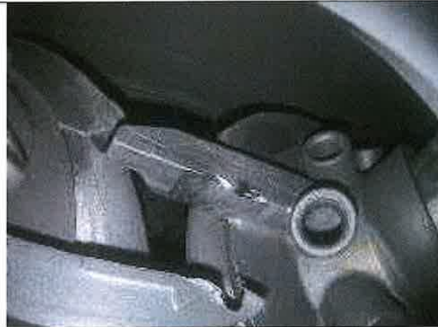
Anti-Rotation Tabs with wear
