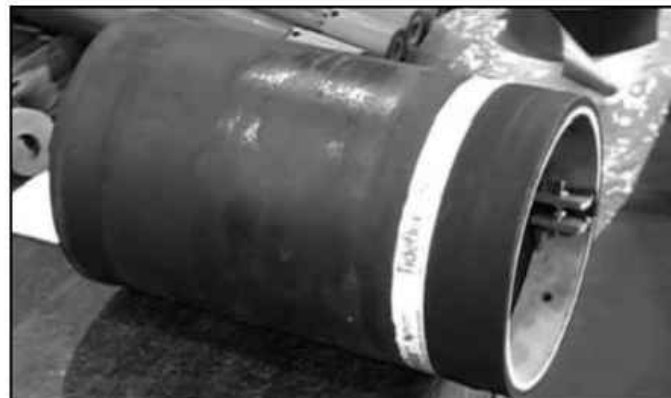
STEP A: Place the valve on a solid, flat surface with the clamped end hanging slightly over the edge of the surface.
