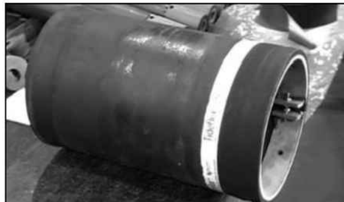
STEP A: Place the valve on a solid, flat surface with the clamped end hanging slightly over the edge of the surface.
