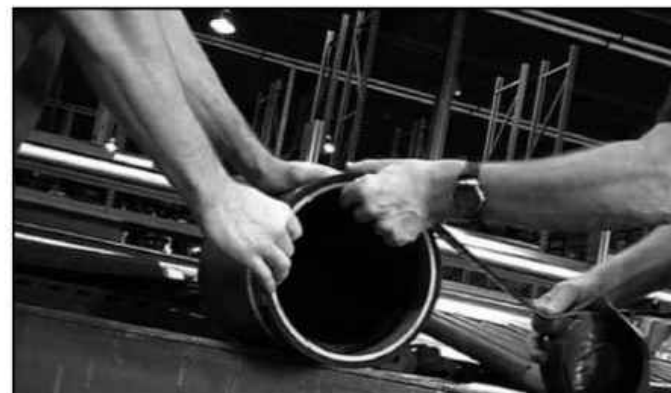
STEP C: Repeat steps A and B on the opposite side of the valve to ensure uniformity of the CheckMate's® O.D. is consistent and matches the pipe I.D.
