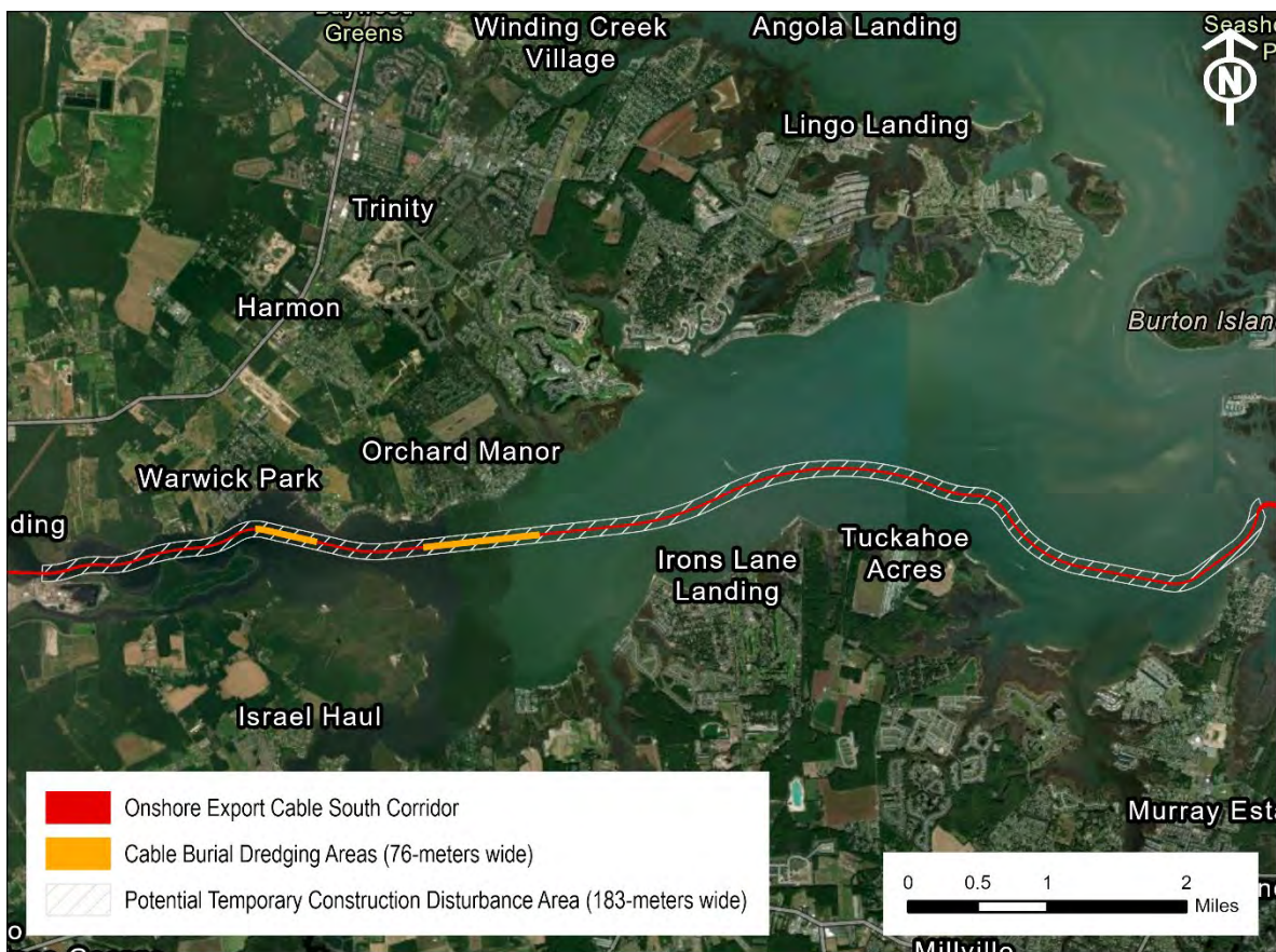
Figure 2-1. Cable Burial Dredging Areas within Indian River Bay
