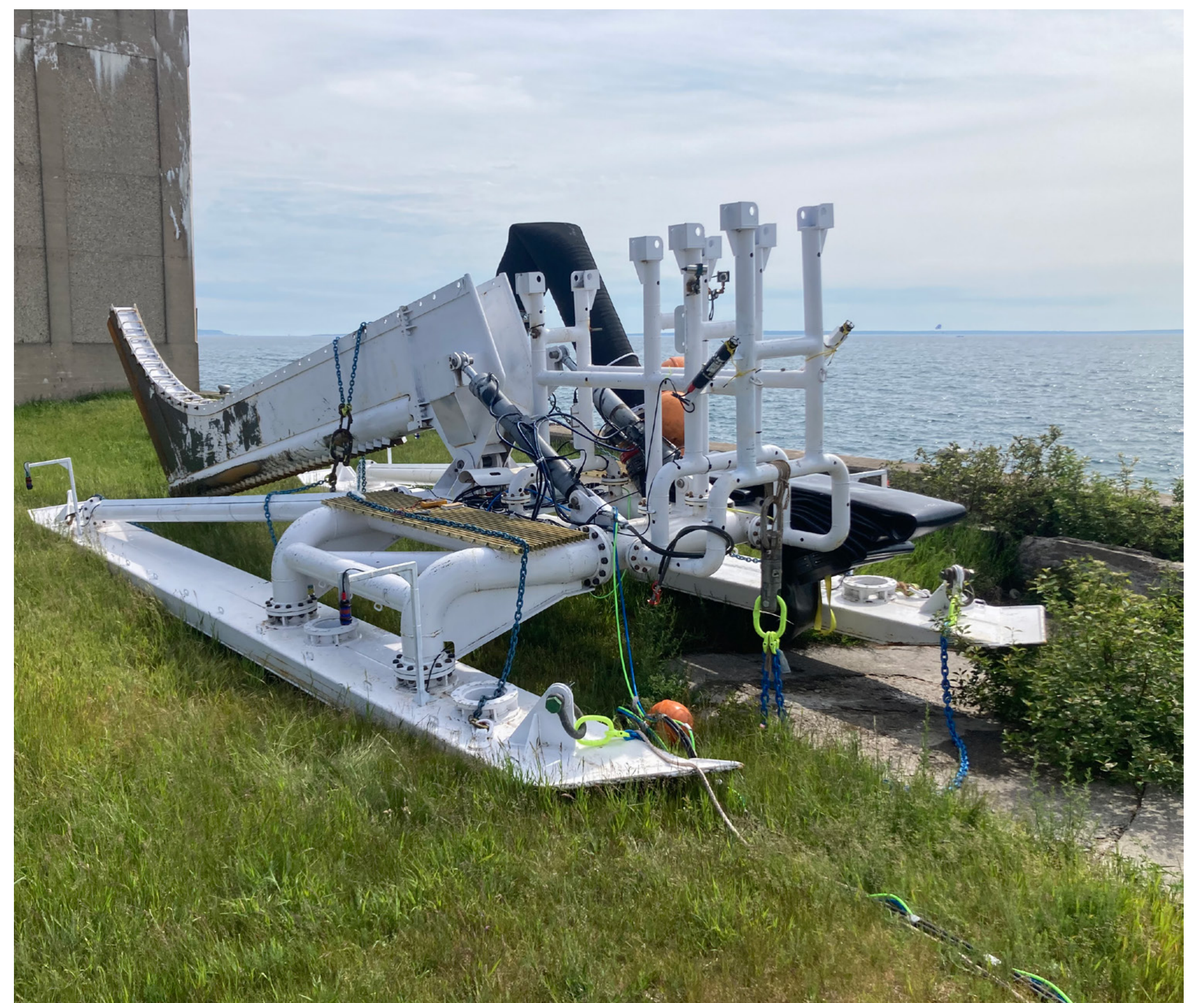
This photo shows a representative Jet Sled used to bury cable in shallow water.
