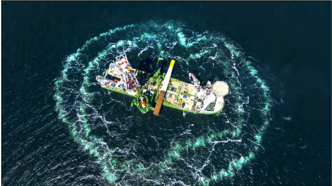
Figure 2. Drone view of the Orion showing double bubble curtains operating. Air compressor support vessel is out of frame at lower left edge of photo. The hydro sound damper is hung around the monopile from sea level to seabed. Photo by DEME [7].
