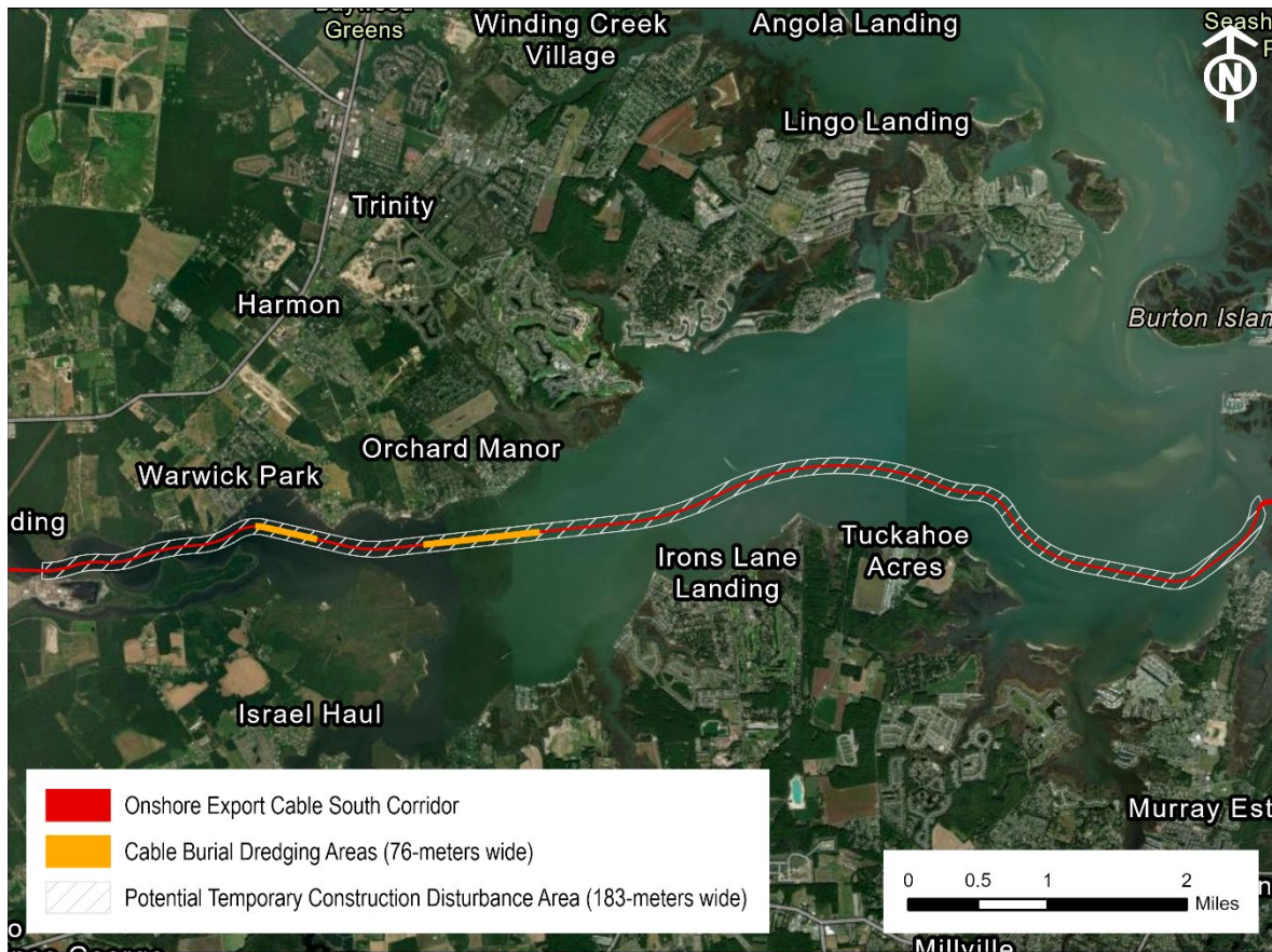
Figure 2.1-16. Cable Burial Dredging Areas within Indian River Bay
