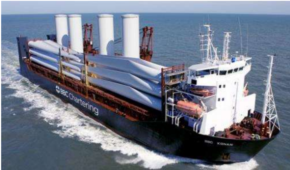
Figure 3.2-12. Tower Sections Onboard the BBC Chartering and Logistic Ship M/V BBC Konan (Source: gcaptain.com)
