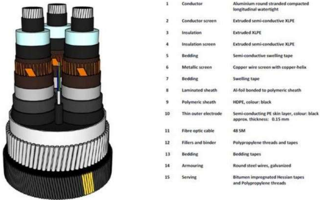
Figure 3.1-10. Inter-array Cable (Source: Nexans)
