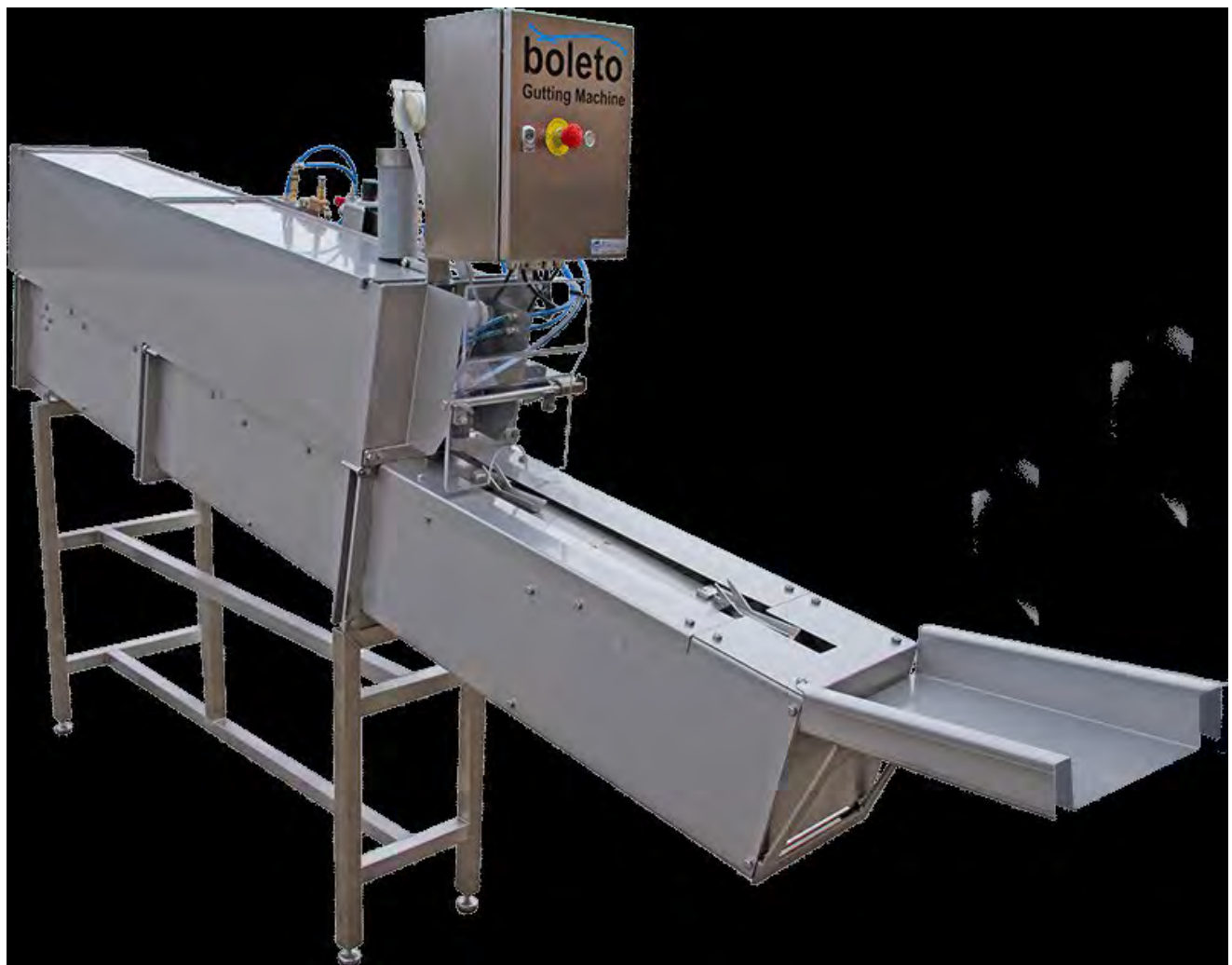
Gutting machine used to remove insides from the fish.
