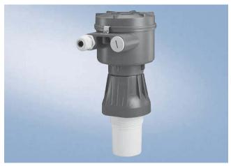
The Pointek ULS 200 is an ultrasonic non-contacting switch with two switch points for level detection of bulk solids, liquids and slurries in a wide variety of industries.
