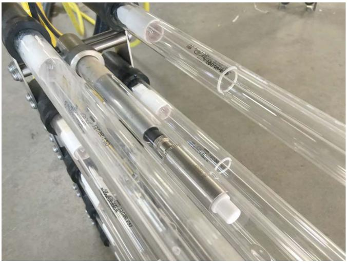
UV sensor is enclosed in its own quartz sleeve
