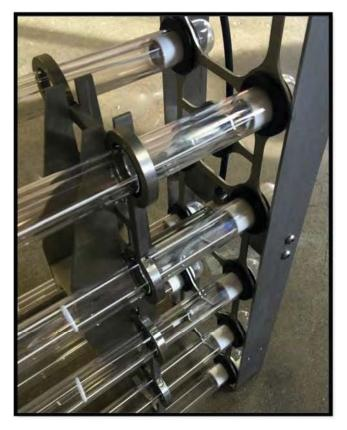
Remove the compression nut. Check to see if the O-ring is inside. Once loosened, take the lamp and slide the end into the quartz sleeve. Make sure that the 4-pin connection remains outside.
