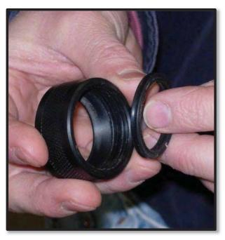
Insert oring into compression nuts
