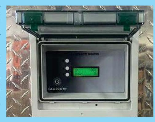
The system is "calibrated" after initial installation of the lamp bank and readjusted after after 100 hour burn in. The monitor is adjusted to indicate 100% for new/clean lamps. Then appropriate operator alert levels are set for the specified decrease in intensity.
