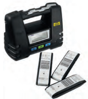
Tube pump Dräger X-act 5000
