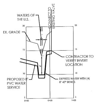
NOTE: UTILITIES SHALL BE BEDDED WITH STONE AND TRENCH WILL BE BACKFILLED WITH EXISTING SOIL TO PREVIOUS GRADE.
