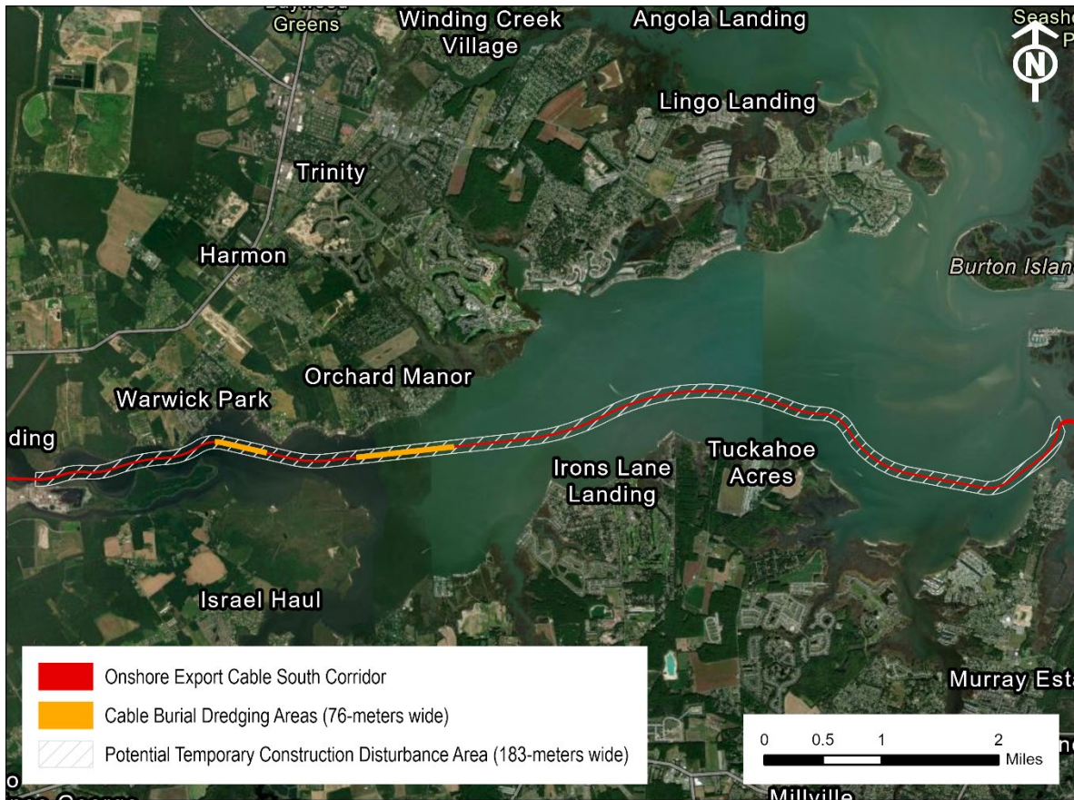
Figure 3. Cable Burial Dredging Areas within Indian River Bay
