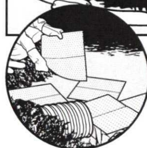
Oil-only absorbents float to confine and absorb spills
