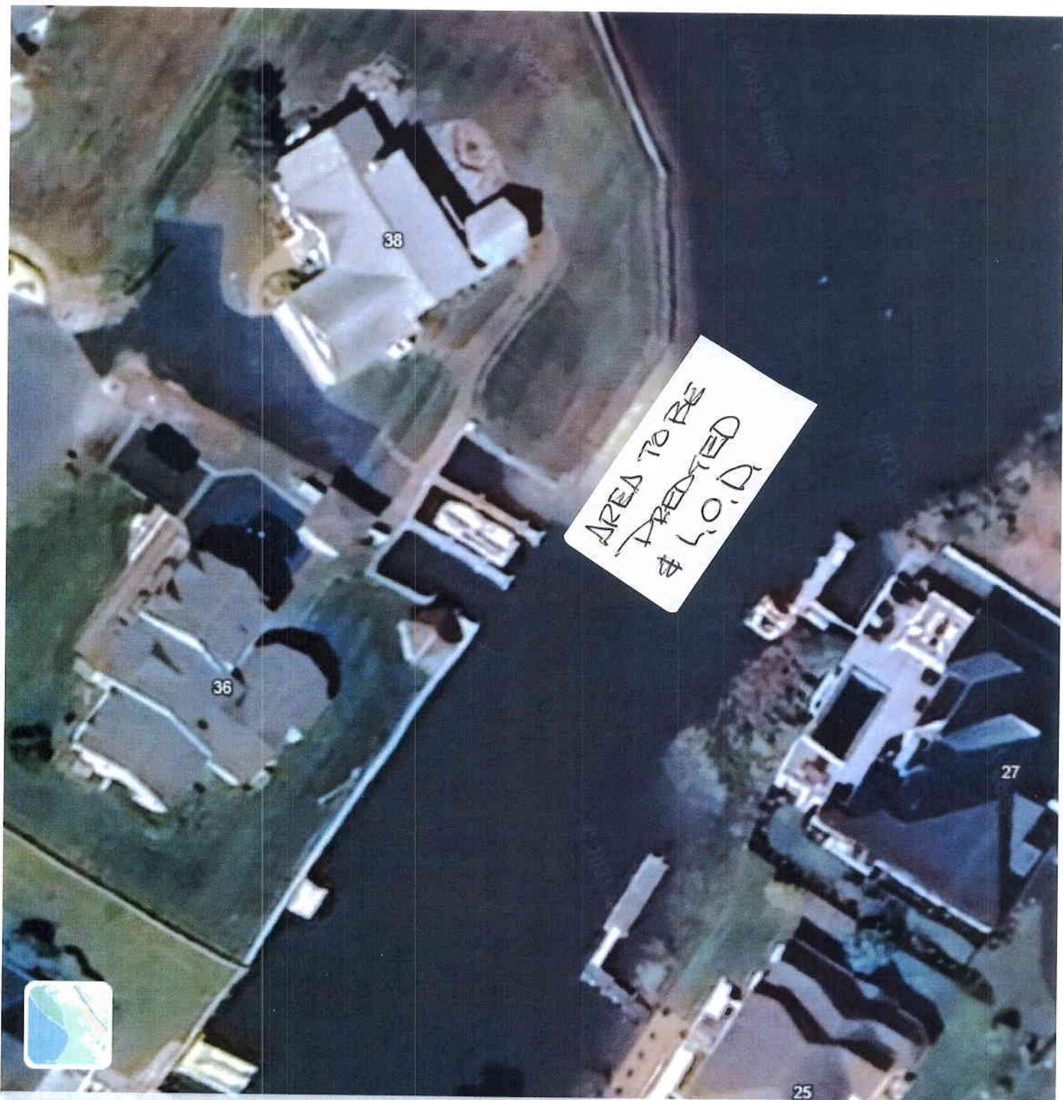
$$70 \text{ FT} \times 5.5 \text{ cu.yds/FT} = 385 \text{ TOTAL cu.yds}$$
