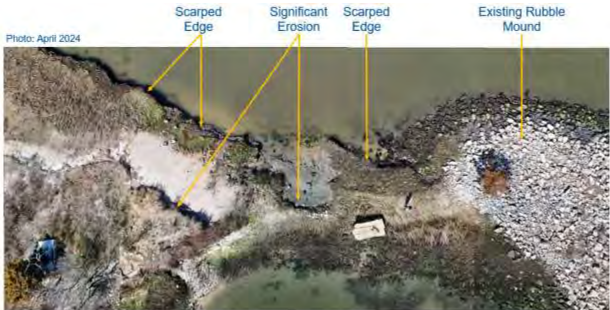
Figure 1. Aerial view of the spit of land showing erosion and scarping.
