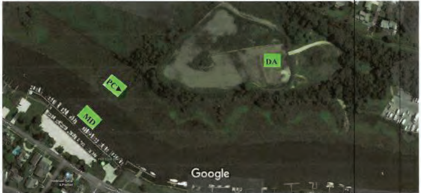
Figure 6. Aerial photograph showing Pilottown Marina (maintenance dredging site, MD), adjacent to Lewes and Rehoboth Canal; disposal area (DA); and pipeline crossing (PC).
