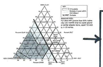
3. Backfill should not have stones greater than 3 inches (75 mm) in diameter or excessive clods that do not break apart during placement and compaction. Backfill must be capable of occupying the spaces between the tank ribs and beneath the haunches.
