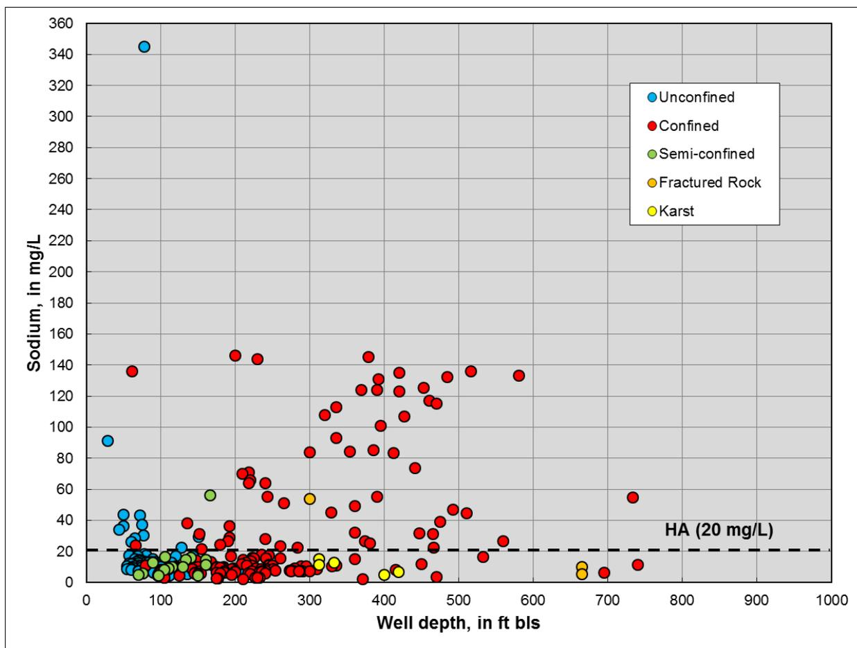
Figure 12. Scatter plot of sodium versus well depth. [mg/L, milligrams per liter; ft bls, feet below land surface; HA, health advisory for public water-supply systems (U.S. EPA, 2012).]
