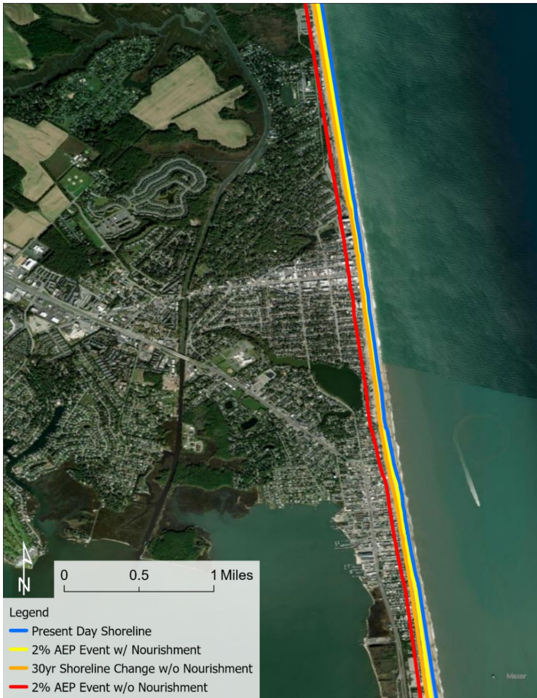
Figure 12-2. Current and future projected shoreline position, as well as shoreline position following a two percent AEP storm event with and without nourishment at Rehoboth-Dewey
