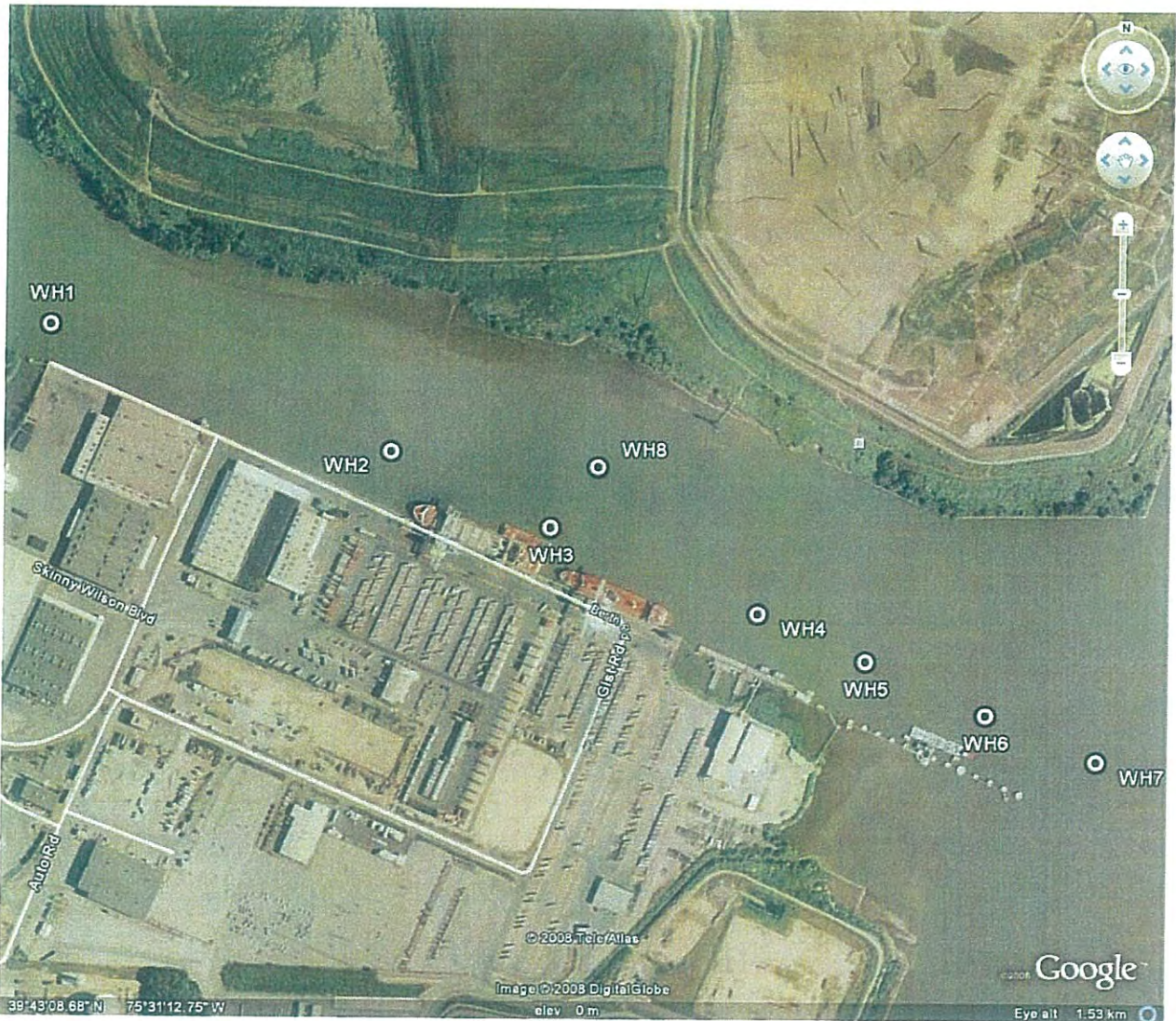
Figure 1. Vibracore station locations for sediment samples taken in June 2008
