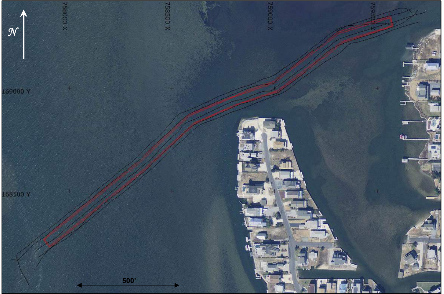
Figure 3. Survey Track Plots – North Channel Survey Area
