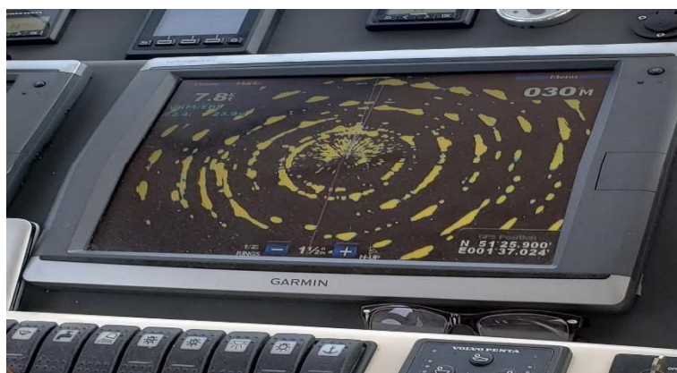
FIGURE 1.3 Photograph of the display of a shipboard radar operated in a U.K. wind farm.
