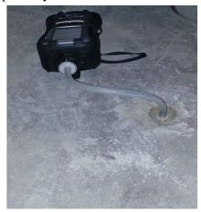
10) To conduct the QA/QC testing and sampling, first connect the hose barb to a length of Teflon-lined polyethylene tubing short enough to fit within a five- gallon bucket and connect the tubing to the hose barb on the top inside of the bucket. When not conducting QA/QC tests or sampling, ensure that the hose barb or stainless-steel tubing is capped.
