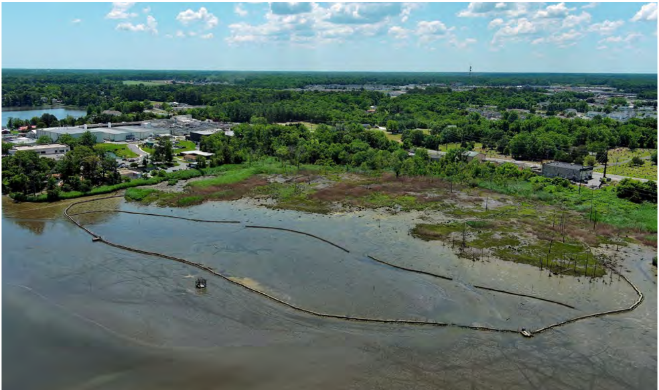
A beneficial use dredging project with a hand-built perimeter designating 15 acres for tidal wetland restoration in the Indian River near Millsboro. PHOTO: DNREC
