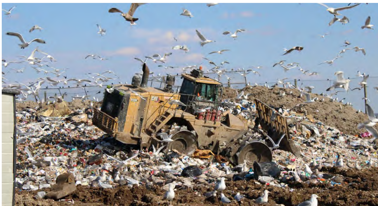
Active face landfill compactor spreading and compressing solid waste. PHOTO: DSWA
