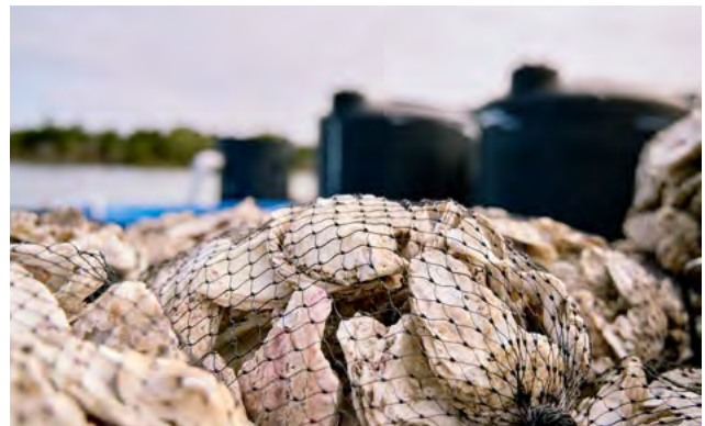
Bagged oyster shells like these are an example of natural materials used in living shorelines. PHOTO: DNREC
