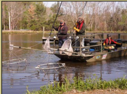
14ft electrofishing boat used to catch game fish to evaluate their populations
