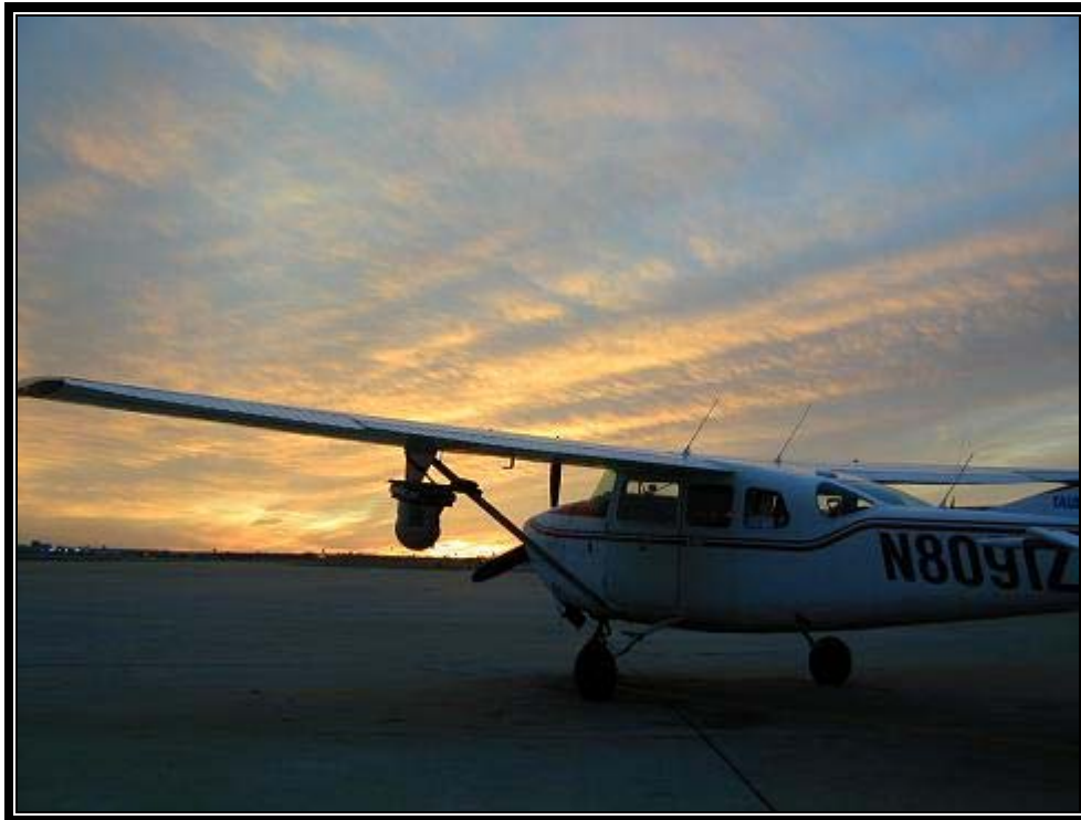
Figure 3. Cessna 206 with Polytech Kelvin 350 II gimbal with infrared sensor mounted on the left wing is used for aerial infrared wildlife surveys.
