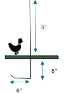
To prevent tunneling into the coop, the fence material should be buried at least 12" deep, or 8" deep with a 90-
