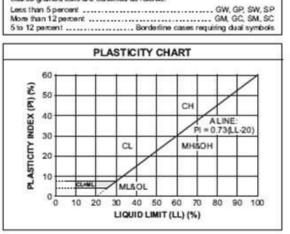
Determine percentages of sand and gravel from grain-size curve. Depending on percentage of fines (fraction smaller than No. 200 sieve size), coarse-grained soils are classified as follows:
